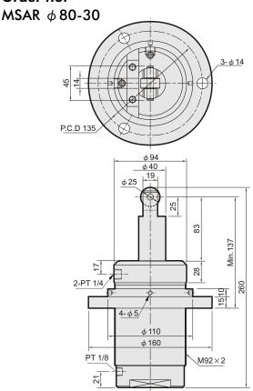
\*\*Roller is made of stainless steel.
