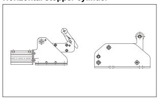
orizontal stopper cylinder of lower height for conveying the heavy work carriers. Suitable as a stopper cylinder for accumulating line, ageing line, and mulit-stage conveyor line. Softly stops the work carriers of heavy weight and high speed.
